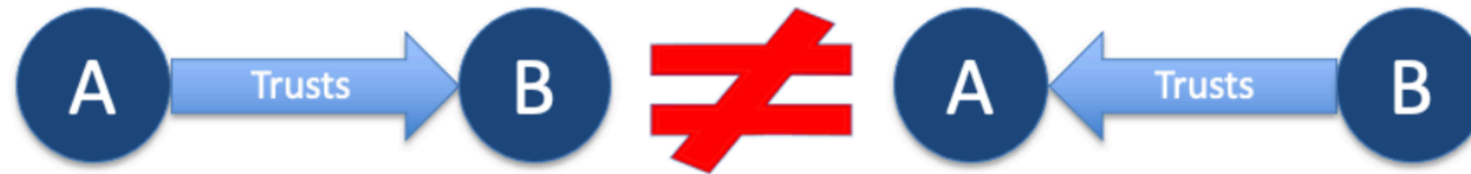
Figure 16. A single trust relationship is always unidirectional. A trust relationship MAY be bidirectional, but if so, it is composed of two unidirectional trust relationships
