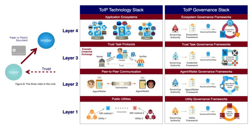
Figure 15. An overview of the four layers and two halves of the ToIP stack
